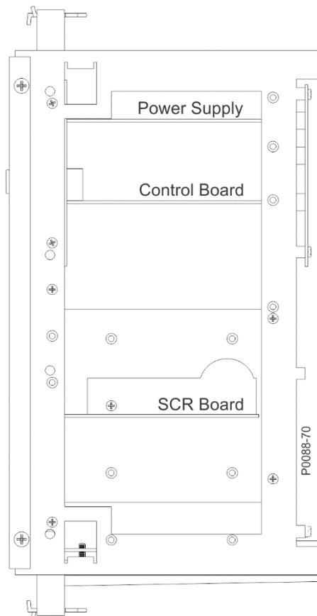
Figure 13. Side View of Cradle Assembly: Circuit Board Locations
