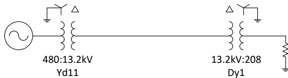
Figure 10. Distribution System Example
